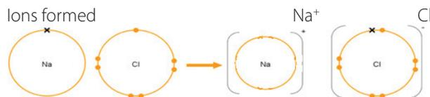
The valence shell electron in sodium is lost, leaving the shell empty while the lost electron is gained by the valence shell of chlorine to attain a maximum number of electrons on a shell.
